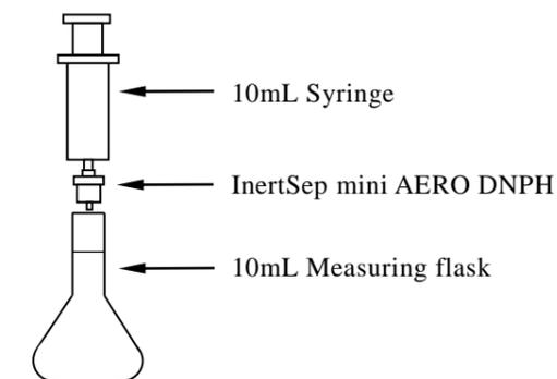
Fig-2 Extraction operation
