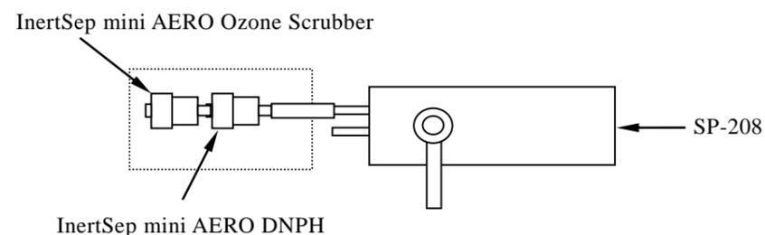
Light shielding ※SP-208 is a sampling pump with flow meter function.
