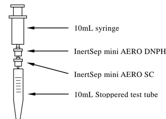
Fig-3 Extraction operation (GC/FTD and GC/MS)
